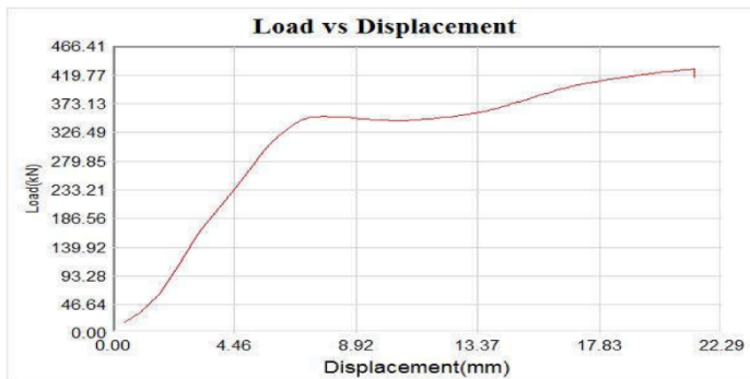
Fig 24 Force-Displacement Curve of Rubber aggregate tube (RUCFST 20%)
