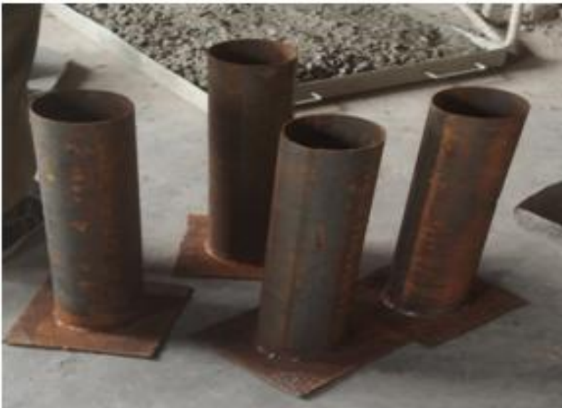
Fig. 6 Circular steel column
