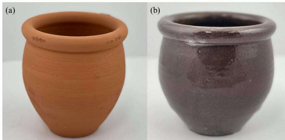
Figure 3 Product of a ceramic plant pot using the raw material composition of No. 5 (calcined at 1,200 °C) with dolomite, Dan Kwian clay, and fly ash of 60 wt%, 20 wt%, and 20 wt%, respectively: (a) before and (b) after coating with clear glaze and firing process.
