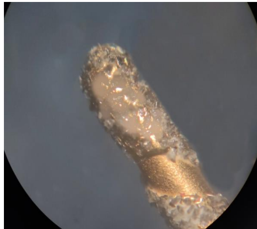
Figure 5: Stereo microscope image of loss of diamond particles on spiral tapered diamond point after repeated cuts with residual diamond particles ( Magnification at 10x)
