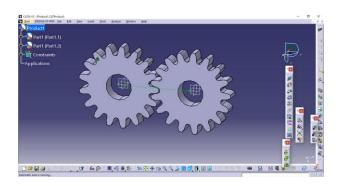
Figure 2 Gear pair assembly model in catia
