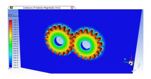
Figure 11 Velocity of Gear at 75 RPM
