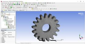
Figure 3 FE Model of a Spur Gear
