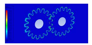
Figure 10 Dynamic Pressure Distributions of Gears under Lubrication
