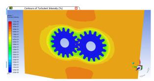
Figure 12 Turbulence of gears under Meshing
