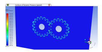
Figure 13 Dynamic Pressure Distribution of gears under lubrication at 75 RPM
