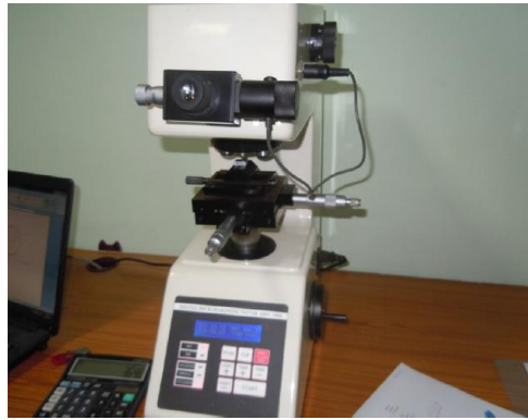
Figure 3 Vickers digital hardness tester DHV-1000
