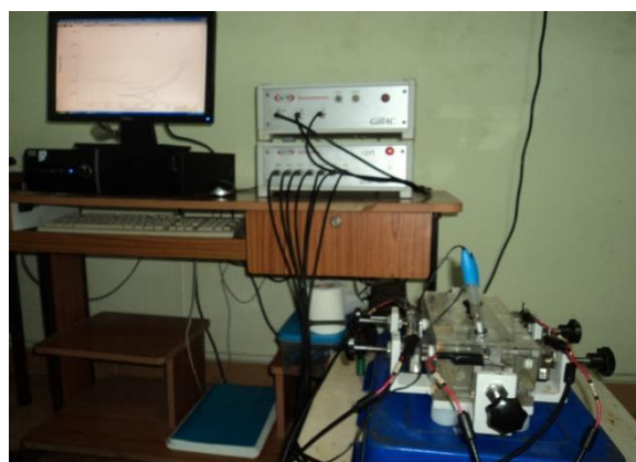
Figure 4 Electrochemical system of GILL AC unit for corrosion test
