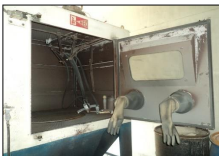
Figure 1 Grit blasting equipment
