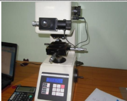
Figure 3 Vickers digital hardness tester DHV-1000
