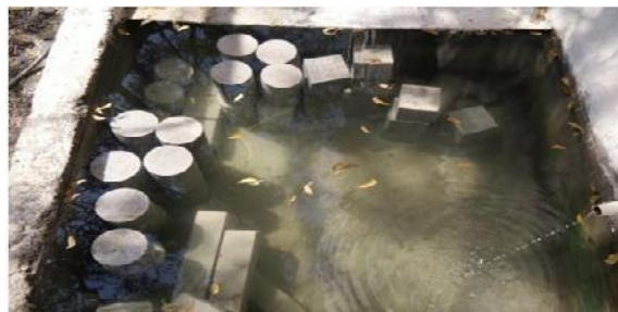
Test specimens kept for curing
