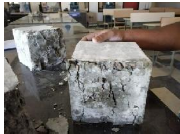
Specimen tested after acid attack
