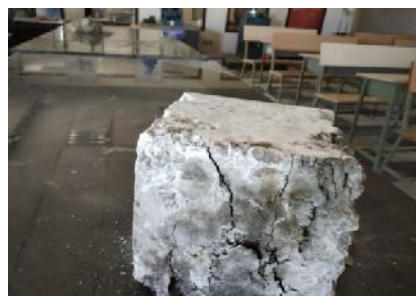
Test specimen after sulphate attack
