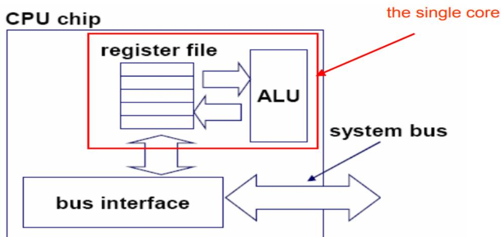
**Fig-2: Archieture of Single Core CPU**
