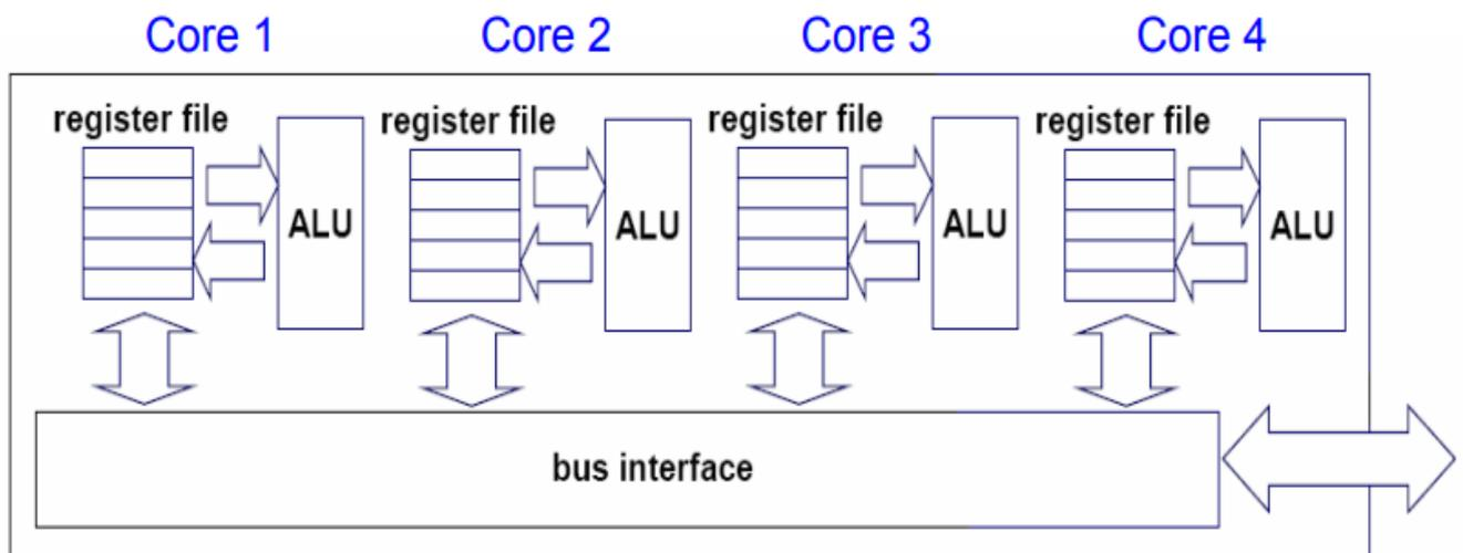
**Fig-3: Architecture of Multi- Core CPU**
